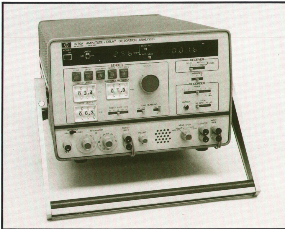
Fig. 1. Model 3770A Amplitude/Delay Distortion Analyzer measures the quality of voice channels used for transmitting digital data. Both the sender and receiver are combined in a single portable unit.
